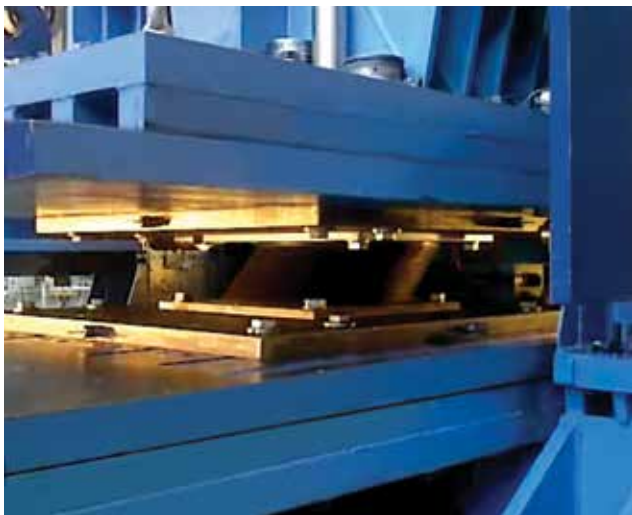
Isolator under dynamic shear deformation testing
