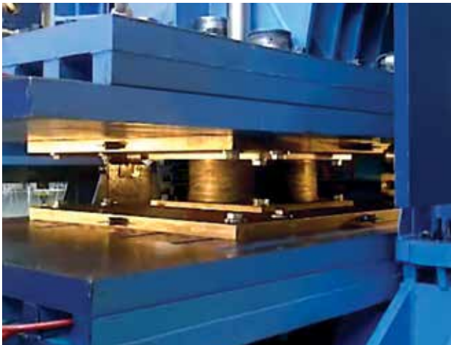
Isolator under dynamic shear deformation testing
